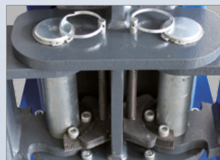
Automatic support-arm restraint with fine adjustment and manual release
