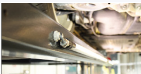
Rotating LED lighting for easy adjustment of light direction for glare free vision.
