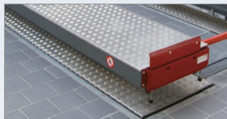
Aluminum clad runways with folded edge for improved water runoff
