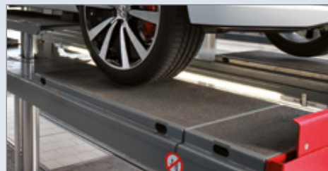
Runways with shims for leveling on wheel-free jacks or for wheel alignment
