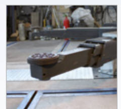
Driveover height on the support disc of 117 mm
