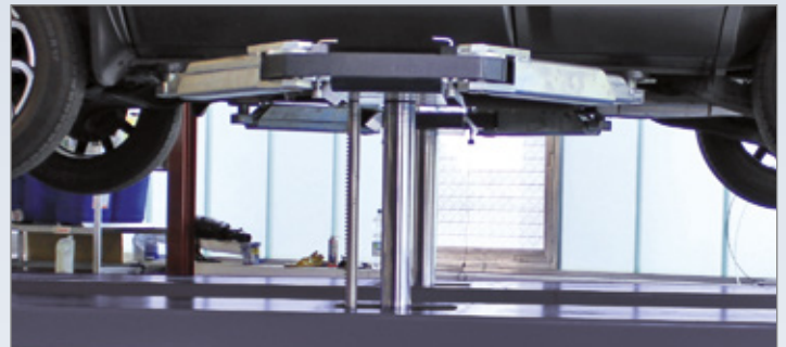
Runway lifts with swing arm wheel-free jack, frame and sill support, load capacity 3.2 t, 3.5 t or 5.0 t
