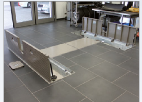
Opening and closing of the cover is supported by a pneumatic damper system
