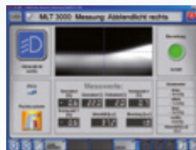
Light test Digital determination of the headlight setting by means of a CMOS camera.
