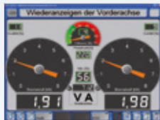
Brake test Digital and graphical display of brake values.
